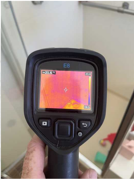
Thermal scan used in conjunction with Tramex moisture meter observed no abnormalities to indicate any live concealed termite nesting at time of inspection.
