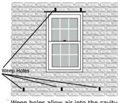
Weep holes allow air into the cavity and moisture to drain out
